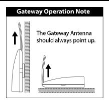
The Gateway should be installed indoors in an easy-to-reach location. Registration requires that you press the gray button on the Gateway. It can be mounted securely to the wall with the included mounting plate and drywall anchors.
